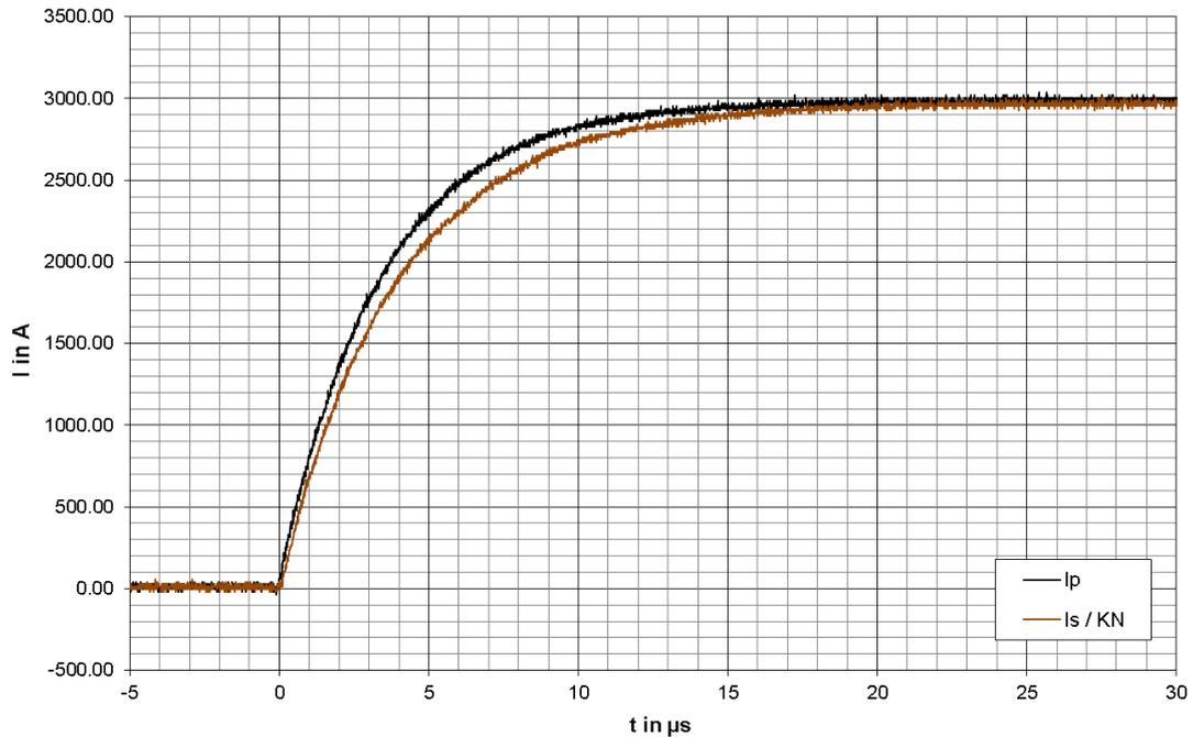
Fig. 2: Output current reaction of a 3kA current pulse with  $R_M = 10\Omega$
