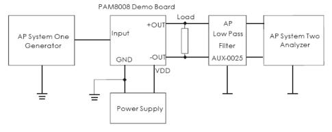
Notes: 1. The AP AUX-0025 low pass filter is necessary for class-D amplifier measurement with AP analyzer.
