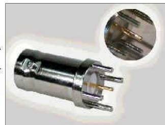
The press-fit center pin locks the connector into the PC board so it is held firmly for reflow or wave soldering.
