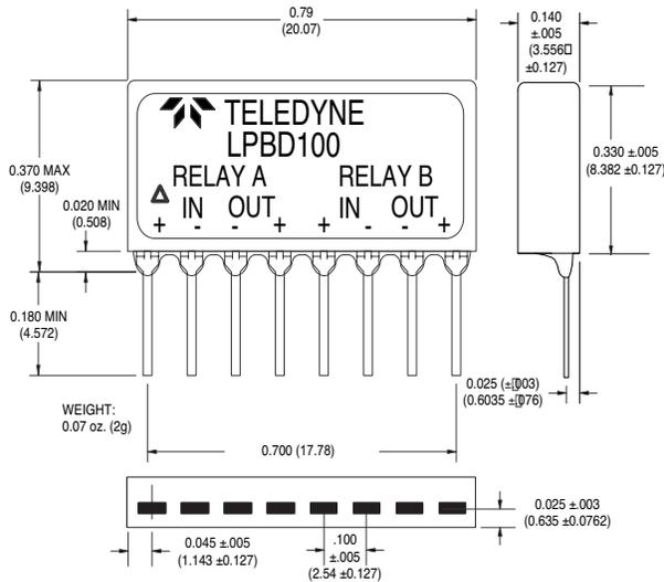
Figure 1 – LPBD100 relay; dimensions in inches (mm)
