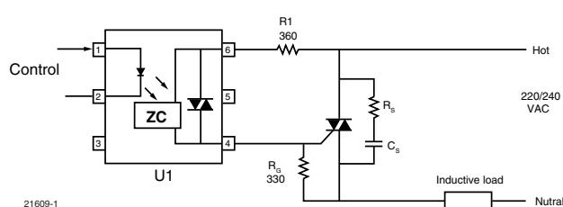
Fig. 12 - Basic Power Triac Driver Circuit
