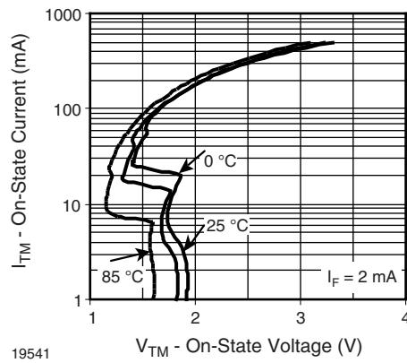
Fig. 5 - On State Current vs. On State Voltage
