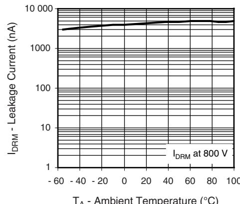
Fig. 4 - Leakage Current vs. Ambient Temperature
