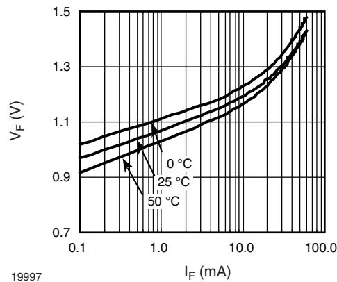
Fig. 2 - Diode Forward Voltage vs. Forward Current
