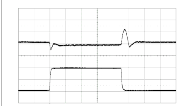
Output Load Transient Response, Default PID/NLR
