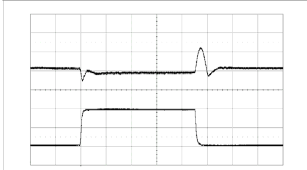
Output Load Transient Response, Default PID/NLR
