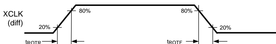
Figure 4. LVDS Output Transition Time
