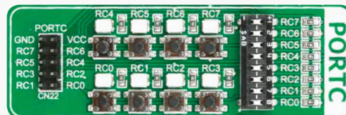
Figure 6-1: I/O group contains PORT headers, tri-state pull up/down DIP switch, buttons and LEDs all in one place
