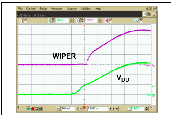
FIGURE 2-14: 2.1 k \Omega – Power-Up Wiper Response Time.
