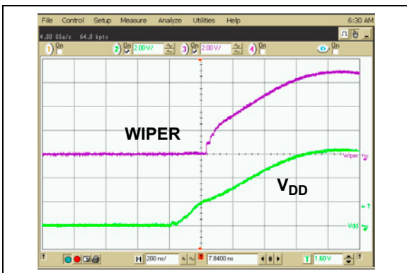
FIGURE 2-14: 2.1 k \Omega – Power-Up Wiper Response Time.
