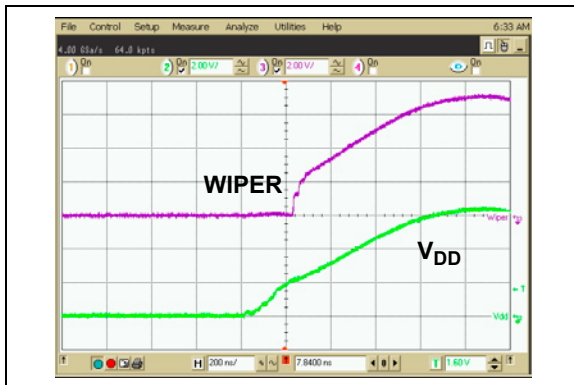
FIGURE 2-45: 50\text{ k}\Omega – Power-Up Wiper Response Time.
