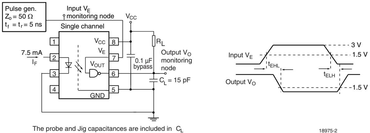
Fig. 3 - Single Channel Test Circuit for  $t_{EHL}$ ,  $t_{ELH}$
