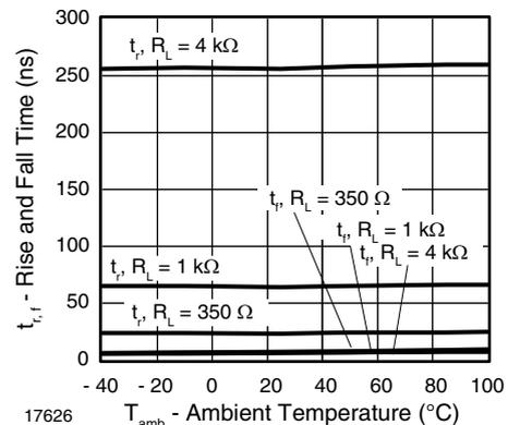
Fig. 21 - Rise and Fall Time vs. Ambient Temperature
