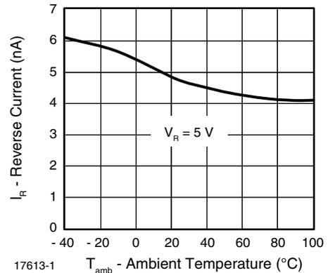
Fig. 8 - Reverse Current vs. Ambient Temperature
