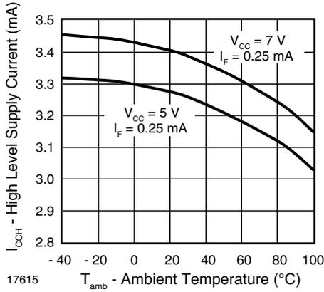
Fig. 10 - High Level Supply Current vs. Ambient Temperature
