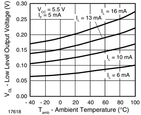
Fig. 13 - Low Level Output Voltage vs. Ambient Temperature
