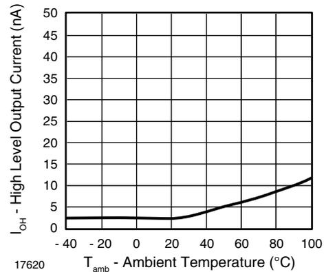
Fig. 15 - High Level Output Current vs. Ambient Temperature
