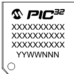
64-Lead TQFP (10x10x1 mm)
