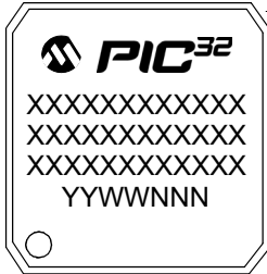
144-Lead TQFP (16x16x1 mm)
