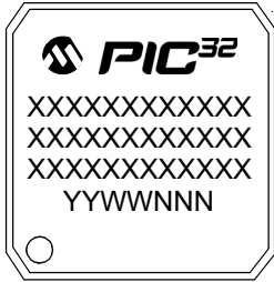
144-Lead TQFP (16x16x1 mm)
