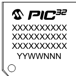
64-Lead TQFP (10x10x1 mm)
