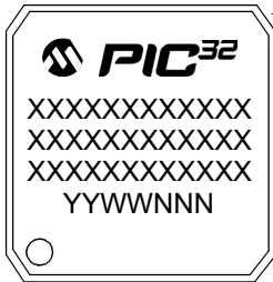
144-Lead TQFP (16x16x1 mm)
