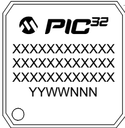
144-Lead TQFP (16x16x1 mm)
