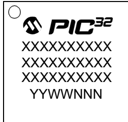
64-Lead QFN (9x9x0.9 mm)
