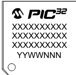
64-Lead TQFP (10x10x1 mm)
