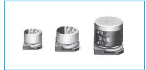
Marking color : Black print (except height : 10mm) White print on a brown sleeve (φ8×10L, φ10×10L)
