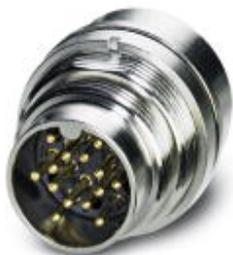
Device connector, rear mounting, straight, Screw locking, M16, number of positions: 8, type of contact: Pin, Solder connection, Axial O-ring, Central fixing, shielded: no
