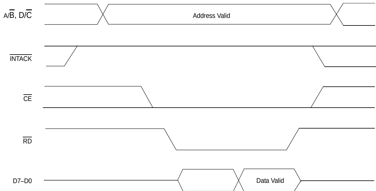
Figure 21. Read Cycle Timing
