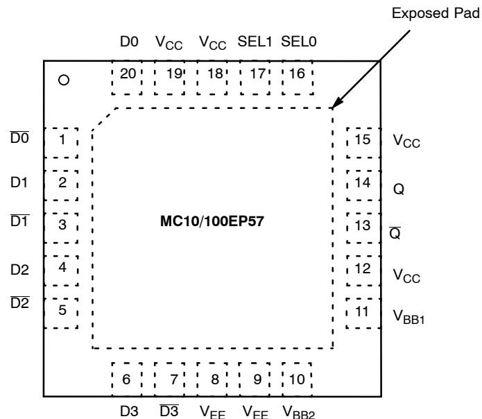
NOTE: The Exposed Pad (EP) on package bottom must be attached to a heat-sinking conduit.
