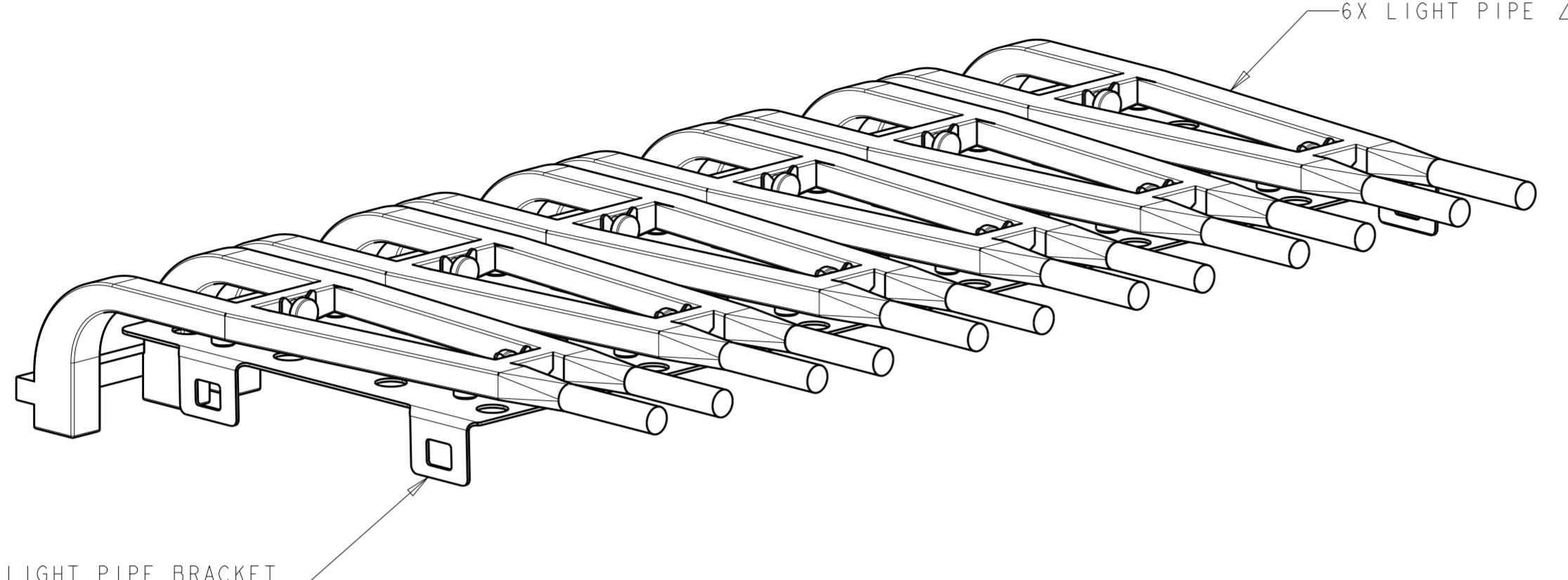
LIGHT PIPE: POLYCARBONATE, CLEAR UL 94V-2
