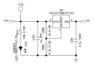
Figure 6. 7.5 V Regulator Schematic
