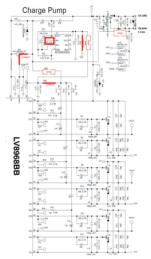
Figure 15. Bootstrap Type Layout of Evaluation Board Schematic
