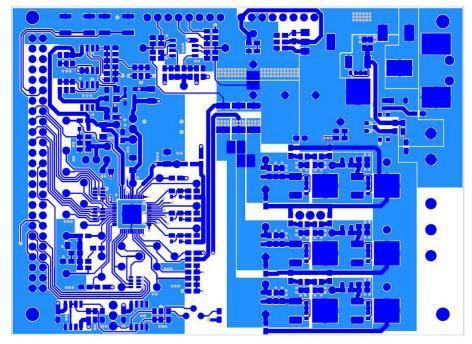
Figure 22. LV8968BB Evaluation Board Layout TOP
