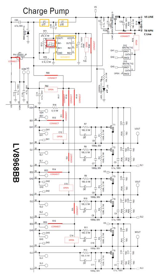
Figure 17. External Charge Pump for 100% Output Duty Cycle Schematic
