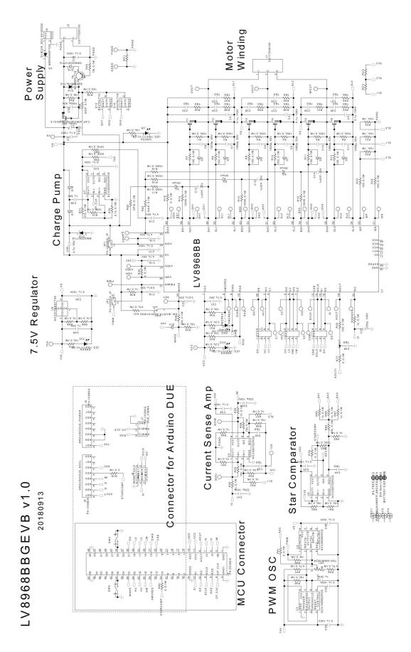
Figure 21. LV8968BB Evaluation Board Schematic
