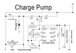
Figure 11. Charge Pump Schematic
