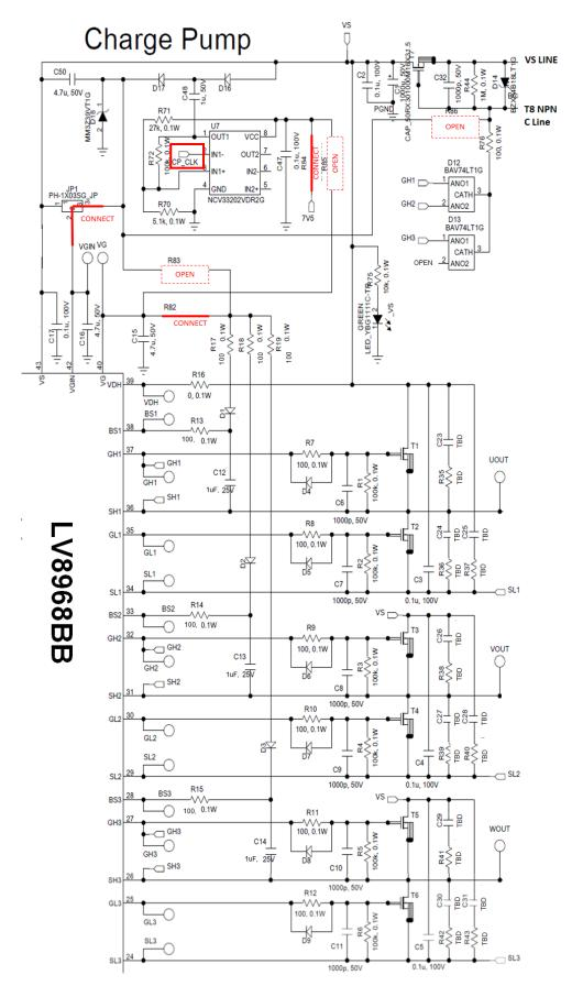
Figure 16. Under Voltage Charge Pump Configuration Schematic
