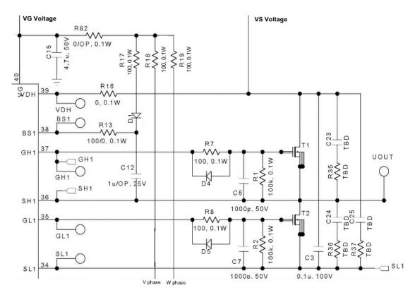
Figure 18. High and Low Side Gate Output Schematic
