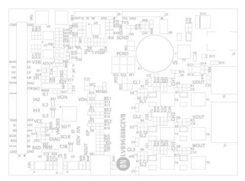
Figure 26. LV8968BB Evaluation Board Layout Silk Name
