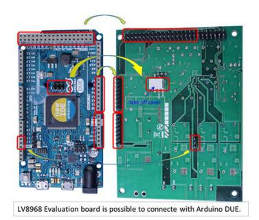
Figure 5. LV8968 Evaluation Board and Arduino DUE
