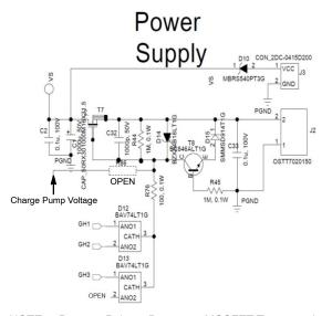
NOTE: Reverse Polarity Protection MOSFET T7 gate voltage is selected by R76 or R86.
