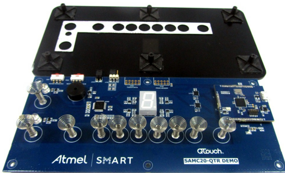
Figure 1-1 Internal View of the Demo Kit
