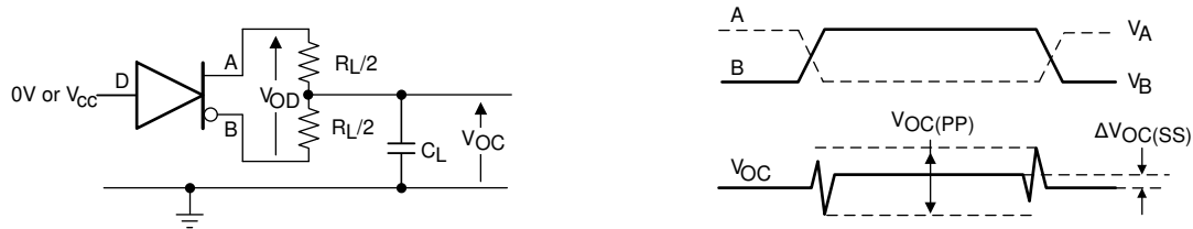
Figure 11. Measurement of Driver Differential and Common-Mode Output With RS-485 Load
