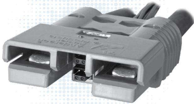
SBX® and SBE® connectors can integrate up to 8 auxiliary power / signal contacts along with the two primary power circuits. SBE® connectors feature an IEC 60950 touch safe housing molded from a chemical resistant PBT/PC blend resin. SBX® are molded from a rugged PC resin and are rated IP20 per IEC 60529.
