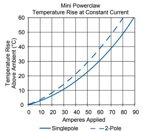
NOTE: Powerclaw charts are based on #8 AWG equivalent copper foil on board side, mated to #6 AWG conductor on wire side.
