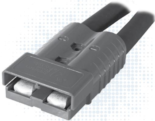
The SB<sup>®</sup>350 is the largest connector in the series with power capabilities up to 450 amps with 4/0 AWG wire and 500 amps with a 350 mcm wire. Wires ranging from #1/0 (53.5 mm<sup>2</sup>) to 350 mcm (150 mm<sup>2</sup>) fit into the one piece housing available in standard PC or a chemical resistant PBT/PC blend. Silver plated wire or busbar contacts minimize electrical resistance while offering supreme durability and reliability.
