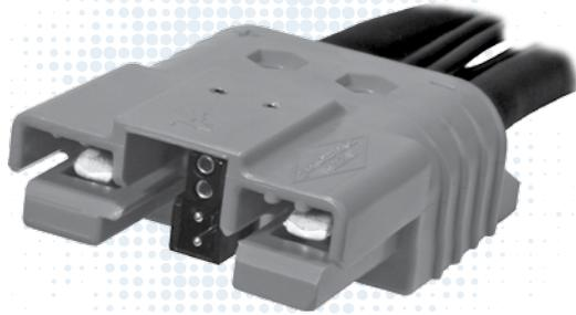
SBE® and SBO® connectors build on the capability of the two pole SB® connectors by offering up to 8 auxiliary power / signal contacts along with an IEC 60950 touch safe housing. The center of the main connector features a connector holder for either: two PP15-45, two PPMX, or APP's innovative 1x4 auxiliary connector.
