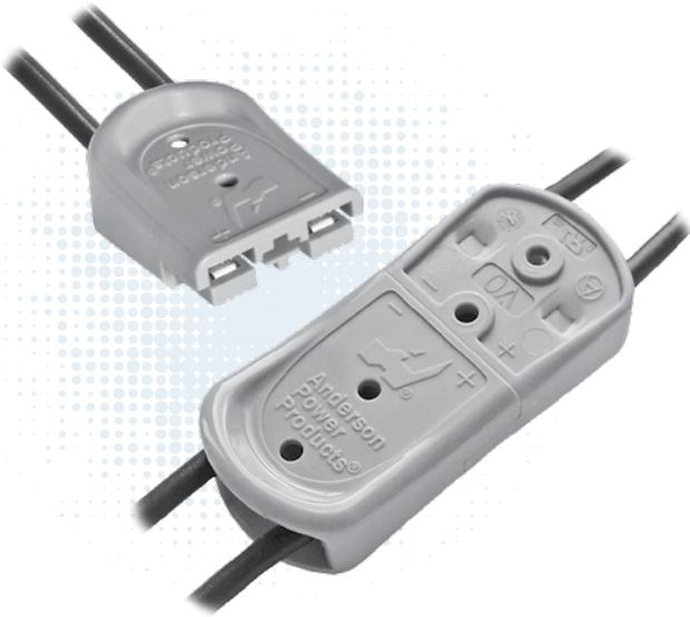
SBS® Mini Connector series is our smallest DC power connector in the SB® group. The SBS® Mini securely holds two crimp and poke contacts with sacrificial tips to enable hot swap capabilities on DC circuits. The low resistance contacts accept 20 to 10 AWG (0.75 to 4.0 mm<sup>2</sup>) wires allowing up to 52 amps of UL rated performance per position.
