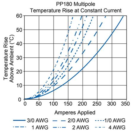
Current - Temperature Derating per IEC 60512-5-2 Test 5B
