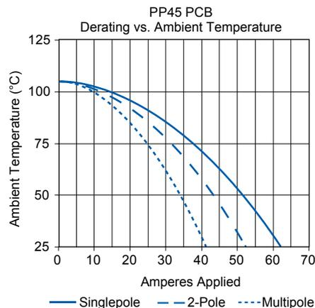
NOTE: PP25 PCB charts based on 0.002 in<sup>2</sup> foil on board side, mated to #12 AWG conductor on wire side. PP45 PCB charts based on #10 AWG equivalent copper foil on board side, mated to #10 AWG conductor on wire side.
