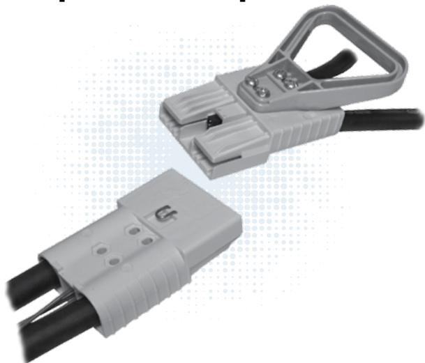
SBX® and SBE® connectors can integrate up to 8 auxiliary power / signal contacts along with the two primary power circuits. Sequencing within auxiliary positions is possible using the 4 pin lengths available in the 1x4 auxiliary connector. The SBE® touch safety rating is equivalent to that of the SBS® connector line.
