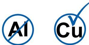
Our connectors are designed to be crimped and/or soldered to multi-stranded copper conductor wires only. Alternate conductor materials including aluminum should not be used. Aluminum conductors crimped into our contacts can result in a galvanic reaction occurring between the aluminum wire and the more cathodic metals used in our contacts including copper, tin, silver, and gold. Additionally softer metals like aluminum flow or loosen from crimps much easier than copper.
