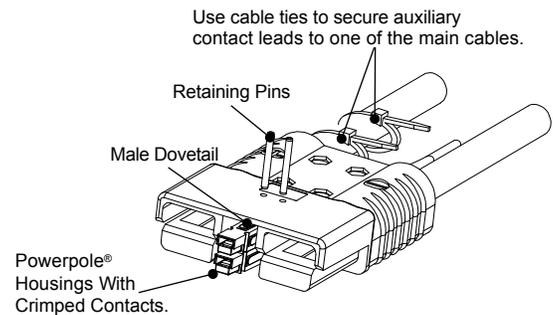
Use cable ties to secure auxiliary contact leads to one of the main cables.
