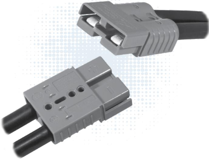
Like the other Multipole connectors, the SB®120 offers color-coded mechanically keyed housings. Keys can be used to identify and separate different circuits, or prevent users from accidentally cross mating different voltages. Wires sizes from #10 (5.3 mm<sup>2</sup>) to #1 (42.4 mm<sup>2</sup>) are held in the second smallest SB® housing.
