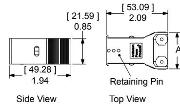
NOTE: Retaining pins are used to secure and position Powerpole® housings in one of three positions in plug shells.
