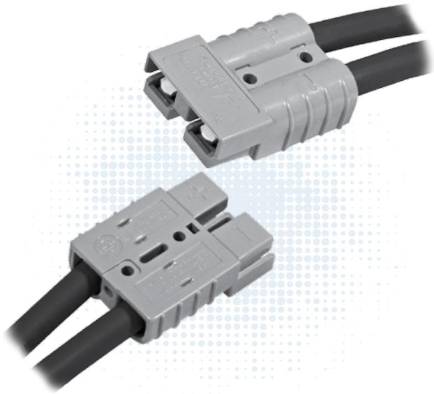
Based off the design pioneered by Anderson in 1953, the two pole SB® connectors set the standard for DC power distribution and battery connections. SB®50 connectors feature a one piece plastic housing using stainless steel springs to hold low resistance contacts in place. Wires sizes from #16 (1.5 mm<sup>2</sup>) to #6 (13.3 mm<sup>2</sup>) are held in the smallest of the SB® series housings.
