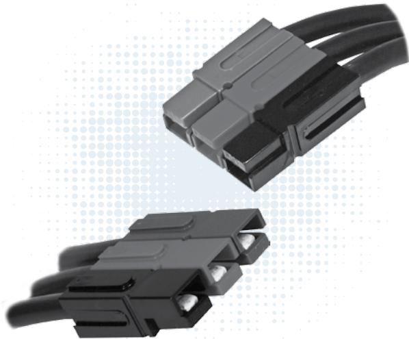
PP120 series Powerpole® housings are designed to accommodate up to 1/0 (50 mm<sup>2</sup>) wires and handle high currents up to 240 amps. Reducing bushings allow PP120 to accept down to #8 (10 mm<sup>2</sup>) wires. Multiple colors of stackable housings combine with low resistance flat wiping technology to offer powerful connection capability.
