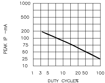
DUTY CYCLE% Fig.6 MAX PEAK CURRENT VS. DUTY CYCLE % (REFRESH RATE f=1KHz)
