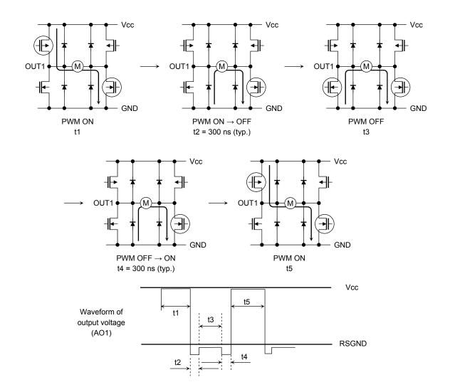
Design target value: Dead time, PWM ON→OFF: t2=300ns PWM OFF→ON: t4=300ns
