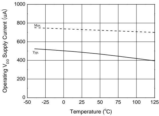
**Figure 12. Operating  $V_{DD}$  Supply Current vs. Temperature**
