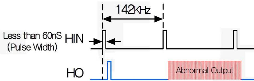
Figure 29. Abnormal Output Waveform with short pulse width
