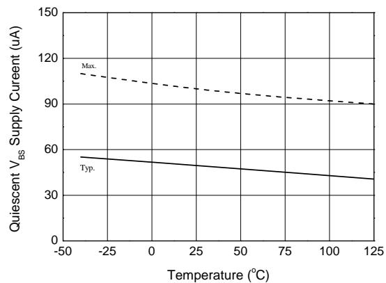
**Figure 11. Quiescent  $V_{BS}$  Supply Current vs. Temperature**
