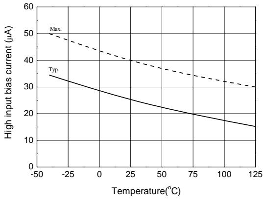
**Figure 22. Logic Input High Bias Current vs. Temperature**
