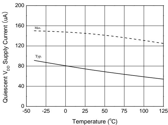
**Figure 10. Quiescent  $V_{DD}$  Supply Current vs. Temperature**
