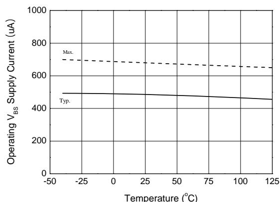
**Figure 13. Operating  $V_{BS}$  Supply Current vs. Temperature.**
