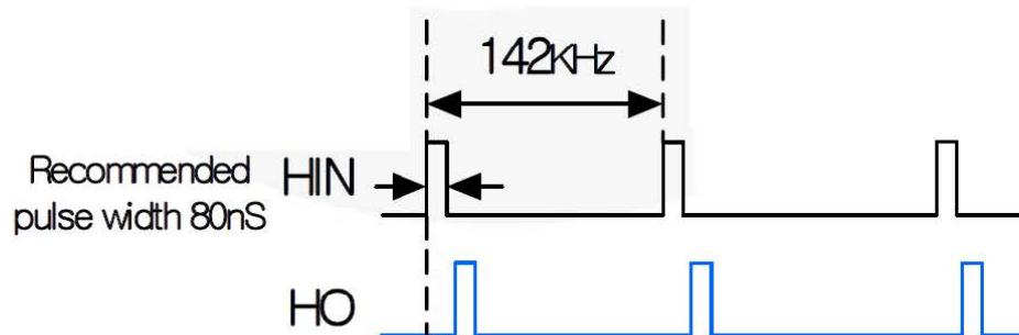
Figure 30. Recommendation of pulse width Output Waveform
