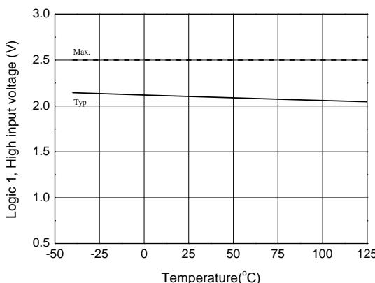
**Figure 20. Logic High Input Voltage vs. Temperature**
