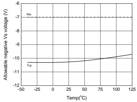
**Figure 23. Allowable Negative  $V_S$  Voltage vs. Temperature**
