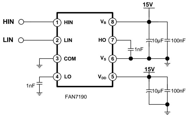
Figure 24. Switching Time Test Circuit (Referenced 8-SOP)
