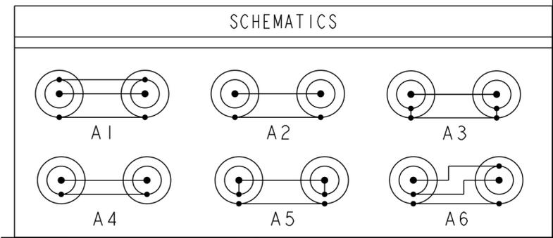
2. WITHIN AND BETWEEN SERIES ADAPTER, MALE CONCENTRIC TWINAX/TRIAX 2/3/4-LUG AND THREADED BAYONET PLUG, TO MALE CONCENTRIC TWINAX/TRIAX 2/3/4-LUG AND THREADED BAYONET PLUG.
