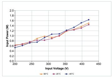
**Figure 3** — Disabled power dissipation vs.  $V_{IN}$
