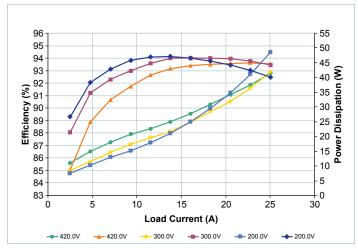
**Figure 13** — Efficiency and power dissipation vs.load at  $T_{CASE} = 25$ °C, nominal trim
