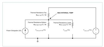
Figure 22 — One side cooling thermal model
