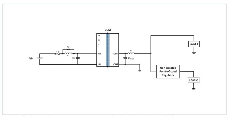
Typical Application 2: Single DCM300P240x600A40, to a non-isolated regulator, and direct to load
