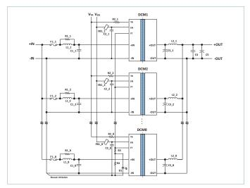
Figure 23 — DCM paralleling configuration circuit 1
