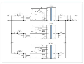
Figure 24 — DCM paralleling configuration circuit 2
