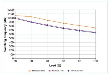
**Figure 18** — Nominal powertrain switching frequency vs. load, at nominal  $V_{\rm IN}$
