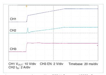
**Figure 17** —Startup from EN,  $V_{IN}$  = 300 V,  $C_{OUT\_EXT}$  = 10000  $\mu$ F,  $R_{LOAD}$  = 0.960  $\Omega$
