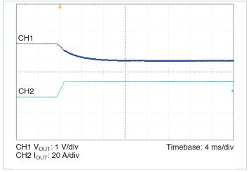
**Figure 8** — 10% to 100% load transient response,  $V_{IN}$  = 300 V, nominal trim,  $C_{OUT\_EXT}$  = 1000  $\mu$ F
