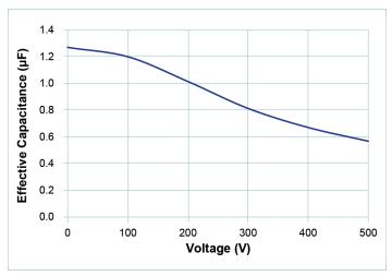
Figure 16 — Effective internal input capacitance vs. applied voltage
