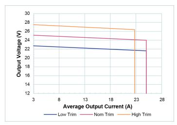
Figure 2 — Electrical Specified Operating Area
