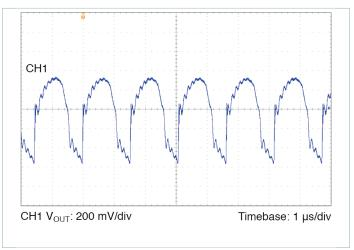
**Figure 19** — Output voltage ripple,  $V_{IN}$  = 300 V,  $V_{OUT}$  = 24.0 V,  $C_{OUT\_EXT}$  = 1000  $\mu$ F,  $R_{LOAD}$  = 0.960  $\Omega$
