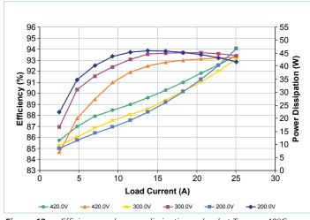
**Figure 12** — Efficiency and power dissipation vs.load at  $T_{CASE} = -40$ °C, nominal trim
