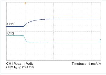
**Figure 7** — 100% to 10% load transient response,  $V_{IN}$  = 300 V, nominal trim,  $C_{OUT\_EXT}$  = 1000  $\mu$ F
