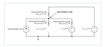
**Figure 21** — One side cooling and leads thermal model
