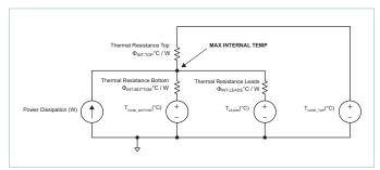
Figure 20 — Double side cooling and leads thermal model
