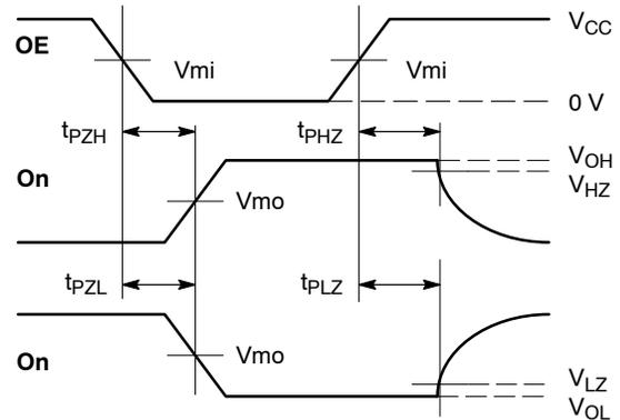
**WAVEFORM 2 – OUTPUT ENABLE AND DISABLE TIMES**
