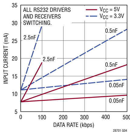
V_{CC} Supply Current vs RS232 Data Rate
