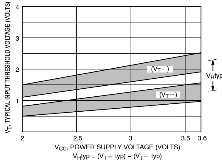
**Figure 5. Typical Input Threshold, V<sub>T</sub>+, V<sub>T</sub>- versus Power Supply Voltage**
