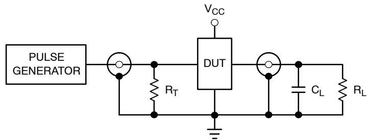
R<sub>T</sub> = C<sub>L</sub> or equivalent (includes jog and probe capacitance)
