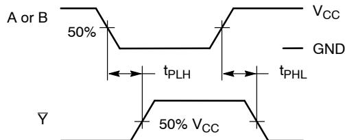
**Figure 3. Switching Waveforms**
