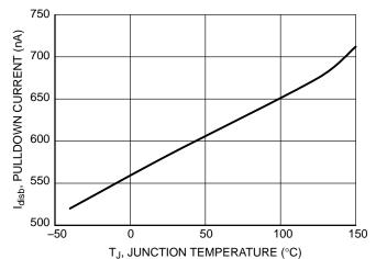
Figure 13. DISB Pulldown Current vs.
