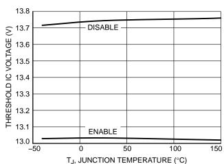
Figure 12. NCV887740 Threshold IC Voltage vs. Temperature
