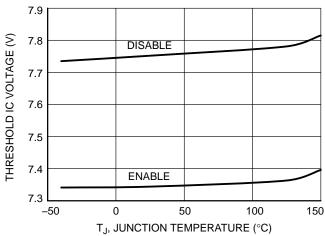
Figure 10. NCV887700/01 Threshold IC Voltage vs. Temperature
