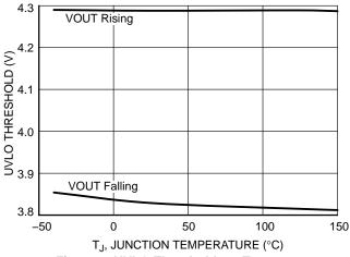
Figure 9. UVLO Threshold vs. Temperature
