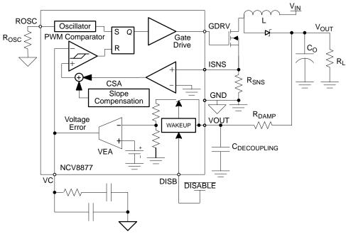
Figure 14. Current Mode Control Schematic
