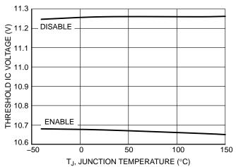
Figure 11. NCV887720 Threshold IC Voltage vs. Temperature
