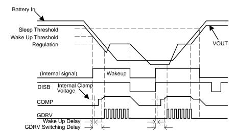
Figure 2. Functional Waveforms
