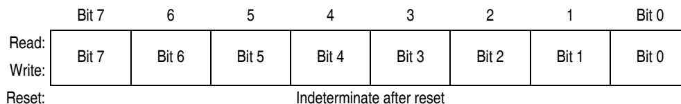
Figure 14-13. TIM Channel Register Low (TCHxL)
