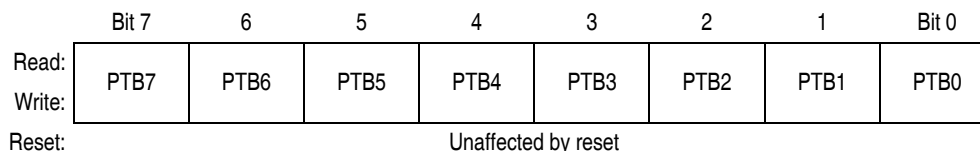
Figure 12-5. Port B Data Register (PTB)
