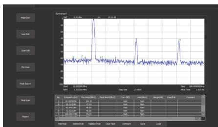
Use the provided EMI software (available for download at [www.bkprecision.com](http://www.bkprecision.com)) to configure the spectrum analyzer, perform prescan, peak search, final scan and generate reports of your pre-compliance tests.
