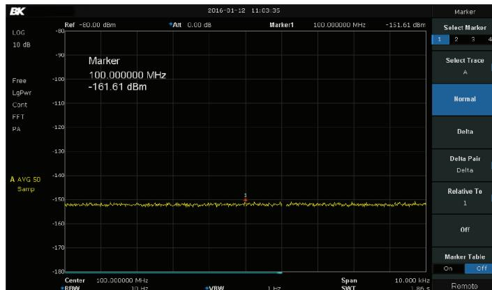
Take advantage of the preamp and -161 dBm DANL to measure low level signals accurately.
