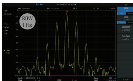
Low resolution bandwidth helps differentiate between adjacent signals
