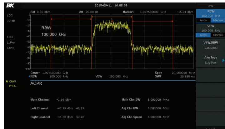
In today's crowded spectrum, ACPR measurements are critical to ensure compliance with regulations. The 2680 series displays the main channel power, left and right channel power as well as bandwidth for each channel on screen for ease of determining the total power being transmitted and the spectrum being used.
