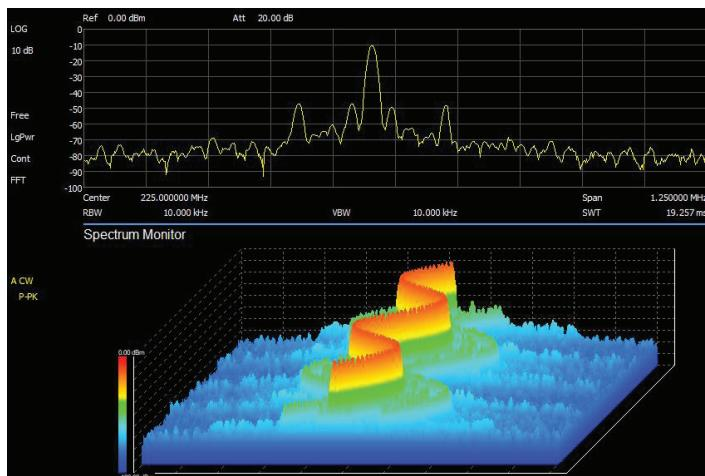
The 2D and 3D spectrum monitor features are standard on the 2.1 GHz and 3.2 GHz models. The 3D spectrum monitor can be displayed using the provided PC software, while the 2D is viewable on the spectrum analyzer screen and in the PC software. This feature shows how the frequency content of a signal changes over time by representing the power intensity with a color gradient.
