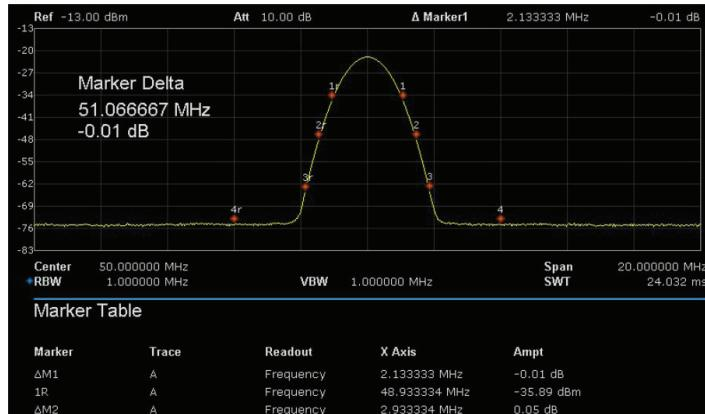
Powerful delta markers can be used to select amplitude, span, stop, start or center frequency, measure noise level, amplitude or frequency.
