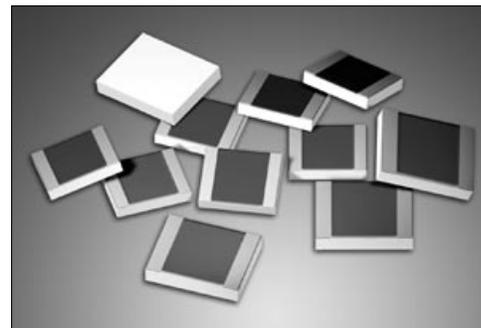
**Style FC - Flip Chip Version** is a surface mount version with solderable pads for flip chip soldering.
