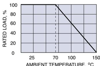
**Note 1: General Applications** - The power rating for general applications is based upon 0.5 sq. in. (300 mm<sup>2</sup>) of termination pad or trace area (2 oz. copper) connected to each end of the resistor. Maximum chip temperature is 150°C. Use Derating Curve to derate appropriately for the maximum ambient temperature and for the temperature limitations of the adjacent materials.
