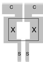
**Fig. 1B:** Kelvin layout recommended for higher resistance values.
