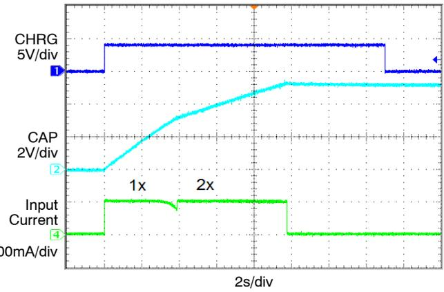
Figure 14. Charge Cycle, 500 mA Input Current
