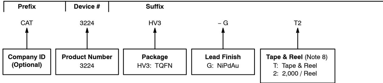
4. The device used in the above example is a CAT3224HV3-GT2 (TQFN, NiPdAu, Tape & Reel, 2,000 / Reel).
