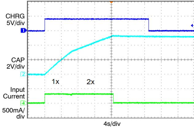
Figure 15. Charge Cycle, 300 mA Input Current
