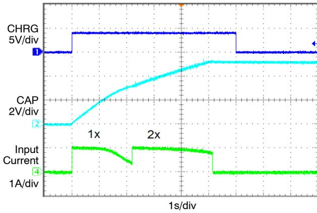
Figure 13. Charge Cycle, 1 A Input Current
