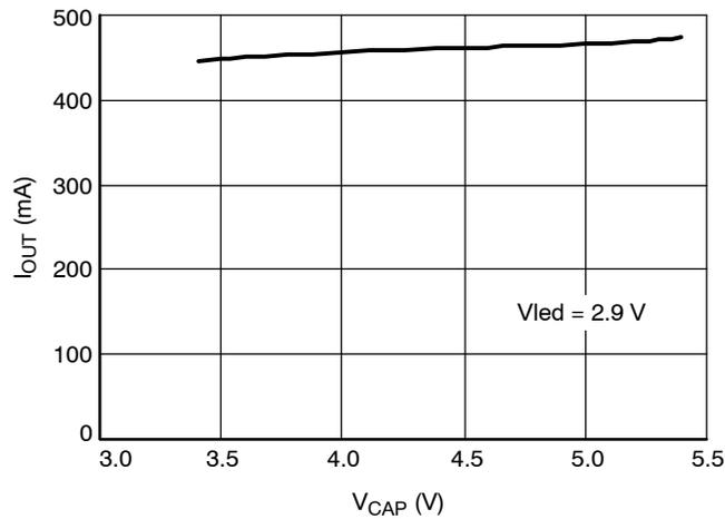
Figure 12. Torch Output Current vs. V<sub>CAP</sub>
