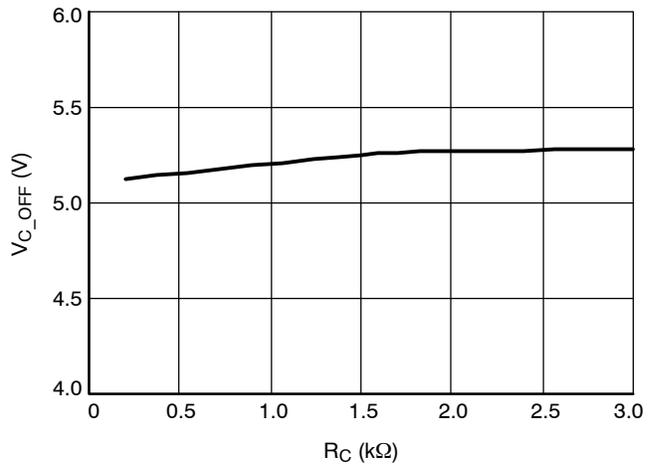
Figure 11. V<sub>CAP</sub> idle vs. R<sub>C</sub>
