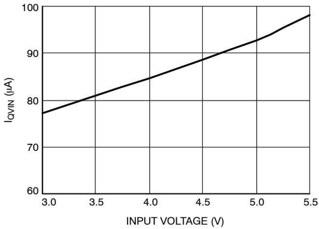
**Figure 3. Idle Quiescent Current vs. Input Voltage**
