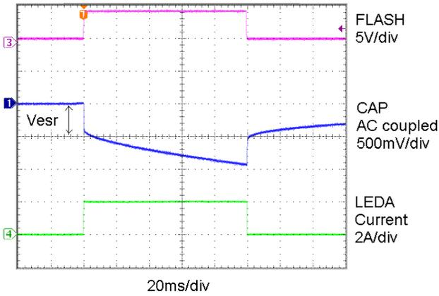
Figure 19. CAP Output Transient during 4 A Flash
