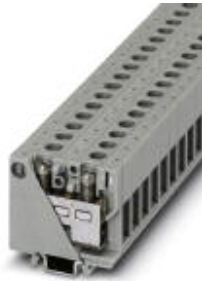
Feed-through terminal block, Connection method: Screw connection, Cross section: 0.5 mm 2 - 10 mm 2 , AWG 20 - 8, Width: 7.5 mm, Color: gray, Mounting type: NS 15
