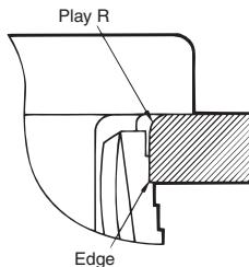
When processing the panel, be sure that the Play R is on the switch operation side.
