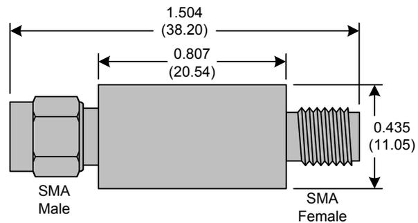
Crystek's new line of High Pass Filters are designed in a rugged SMA housing. This filter line has excellent out-of-band rejection. Designed for Test Equipment and General Lab Use.
