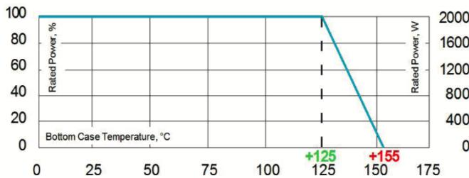
Derating (thermal resist.)FPA2K:  $66.6 \text{ W/K}$  ( $0.015\text{K/W}$ )
