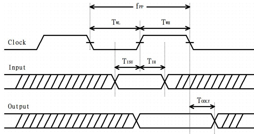
Figure 2: SDIO protocol timing diagram--- default mode (3.3V)
