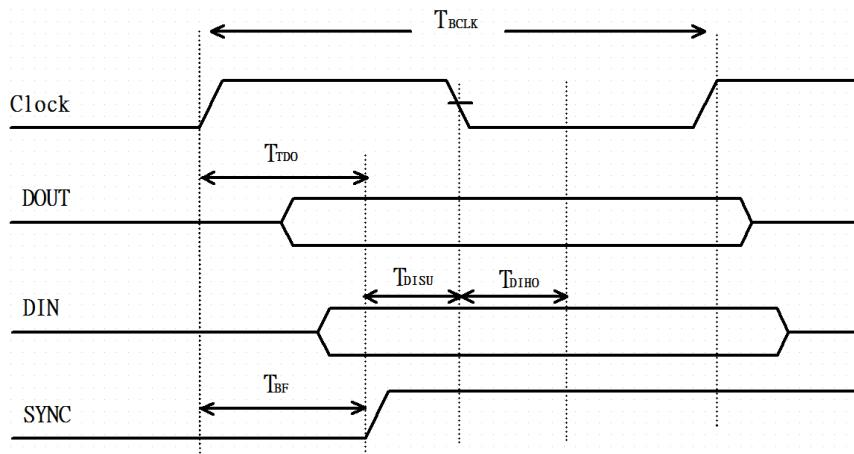
**Figure 8: PCM Timing Specification – Master Mode**
