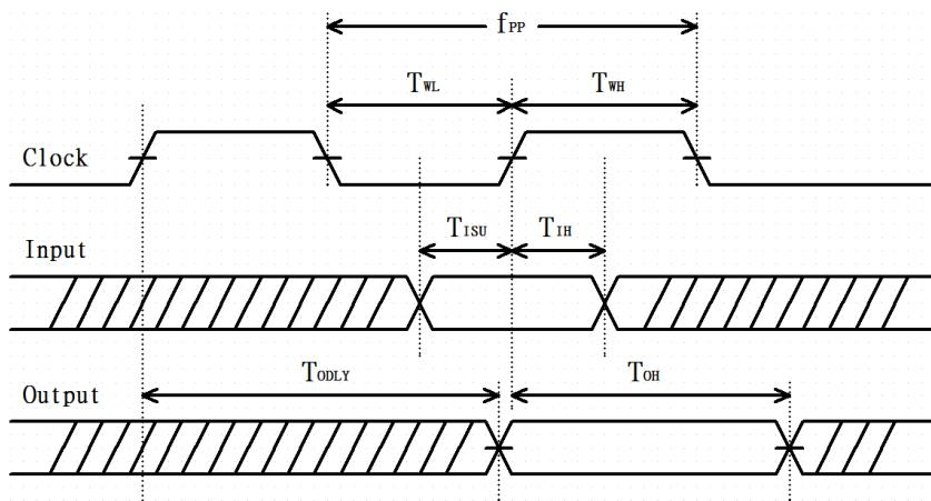
Figure 3: SDIO protocol timing diagram--- High-Speed mode (3.3V)
