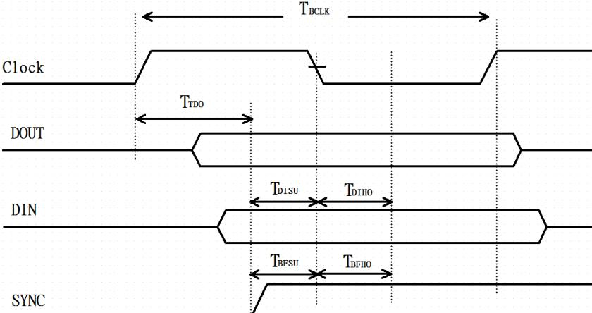
The diagram illustrates the PCM Timing Specification – Slave Mode. It shows four signals over time: Clock, DOUT, DIN, and SYNC. The Clock signal is a square wave. The DOUT signal is sampled by the Clock. The DIN signal is latched by the Clock. The SYNC signal is asserted during the sampling and latching phases. Various timing intervals are labeled: T\_BCLK (clock period), TDO (DOUT-to-Clock), TDISU (DIN-to-Clock), TDIHO (DIN-to-Clock), TBFSU (SYNC-to-Clock), and TBFHO (SYNC-to-Clock).
